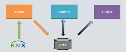
The Recording module uses any KNX interface (USB, IP, also with KNX Security) to record and store KNX telegrams reliably and permanently in the background without supervision. The module runs on Windows or Linux.
